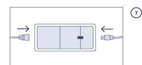
Plug the loose end of the input power cord into the adapter. Plug the wall power cord into the other end of the adapter. We recommend the use of a surge protector (not included) before plugging the cord into your wall.
