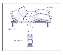
Pair Remote A to Base B, then Base A and Base B can be simultaneously operated by remote A.
